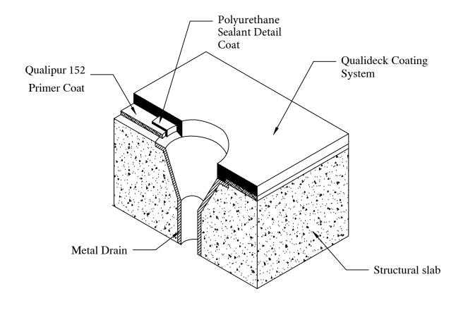
Disclaimer - This detail drawing is intended as a general reference for the condition shown. It is not a specific solution for conditions experienced in the field. To identify specific materials and mil thickness, refer to the Qualideck application guide.
